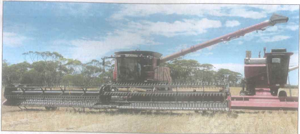
□ The massive Case IH 7240, equipped with a 13.6m (45ft) front dwarfs the International Harvester 711 with a 6m (20ft) front.
